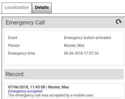
Illustration 24: Emergency call processing with display of detailed information
