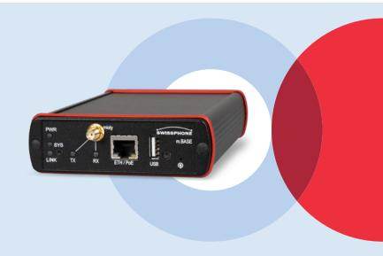
Swissphone's mioty® base station is designed for mission-critical IoT applications that require an optimal bidirectional communication with end-points and sensors. The compact form factor and the high performance RF frontend contribute to its versatility; its redundant power supply architecture with Power over Ethernet (PoE) and two DC inlets make it stand out. The base station offers various hardware variants to meet your requirements.
