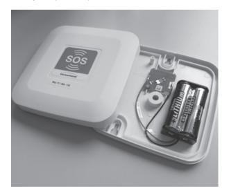
Put the lid back on the base and screw it from below with the screw that you removed before.
